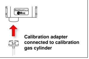
When "CAL" and "go" arer displayed in alternation, and "ZERO" is shown, the instrument is ready to perform a zero calibration.
