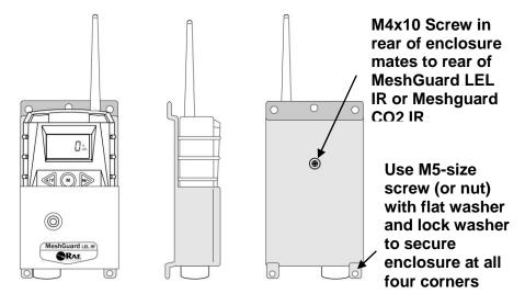
Front, side, and rear views of the steel enclosure show how the instrument is secured for mounting.
