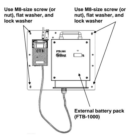
**Note:** The plate holding the battery pack and MeshGuard LEL IR must be mounted on a solid, flat surface.
