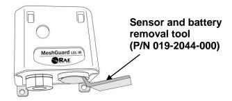
**WARNING:** Use only RAE Systems battery P/N 500-0111-000 (EVE ER34615 or XENO XL-205F) for the internal battery. The internal battery must be replaced under a Hot Work Permit, where the atmosphere is determined to be non-hazardous while the battery is being replaced.
