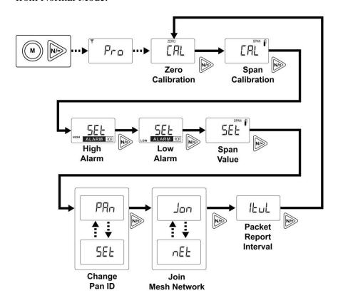
**Modify Span Gas Value.** This function allows selection of the gas concentration to the settings, press [MODE] to repeat stepping through the choices.
