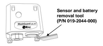
**WARNING:** Use only RAE Systems battery P/N 500-0111-000 (EVE ER34615 or XENO XL-205F) for the internal battery. The internal battery must be replaced under a Hot Work Permit, where the atmosphere is determined to be non-hazardous while the battery is being replaced.
