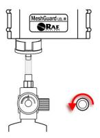
When the gas flow starts, the LCD displays "gAS" and the span concentration value.
