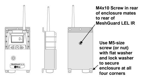
Front, side, and rear views of the steel enclosure show how the instrument is secured for mounting.
